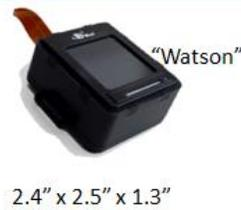
When an electric field is applied across the LES film, and a finger is placed on the film, the EL particles suspended in the film glow beneath the finger resulting in a high resolution image of the fingerprint. That image is in turn captured with conventional camera techniques, and then sent on via a USB 2.0 interface to the host PC, Tablet or Smartphone it is connected to.
